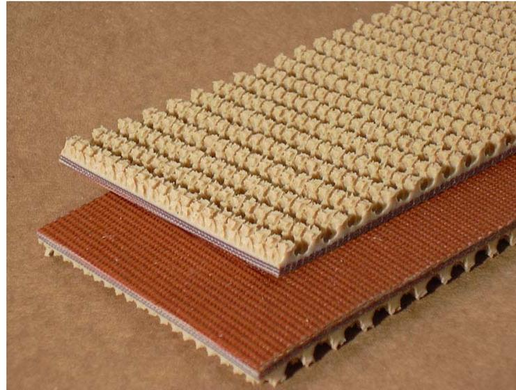
**Features:** 3-1406 offers one of the highest coefficients of friction for steep inclines. This belt cushions the conveyed product with a non-marking surface. NOTE--The Rough Top impression must be recessed to use the recommended lacing. Use Recessed OAG for Lacing Recommendation.
